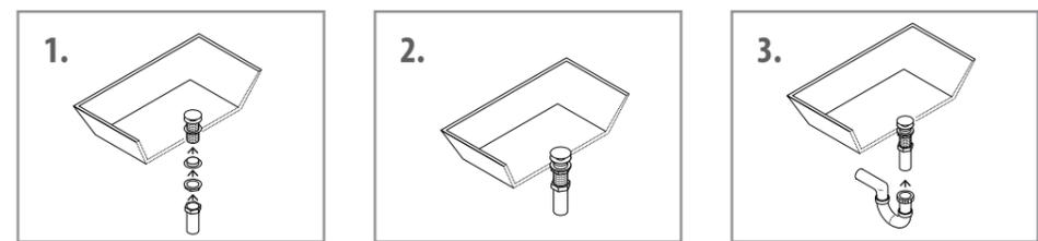
1. After installing the counter top on the cabinet, put the drain assembly inside the hole in the sink and fix it firmly.
