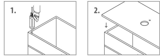
1. Apply continuous stream of quality silicon glue to the top of the cabinet where the glass countertop needs to be placed.
