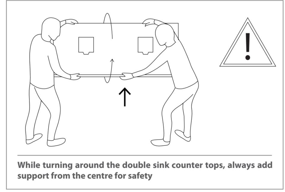
**While turning around the double sink counter tops, always add support from the centre for safety**
