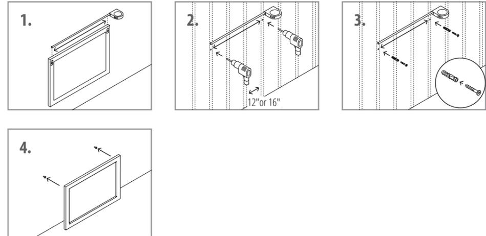
1. Measure the distance between the screw holes from the back of the mirror.
