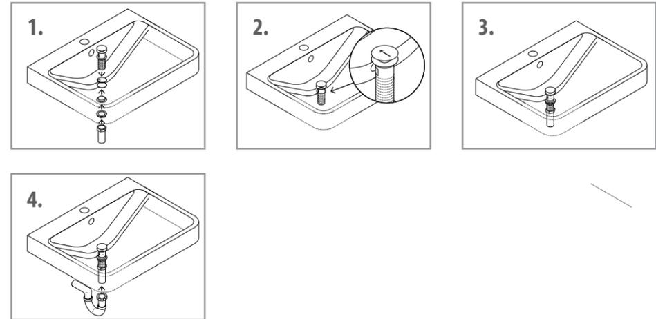
1. After installing the counter top on the cabinet, put the drain assembly inside the hole in the sink and fix it firmly.
