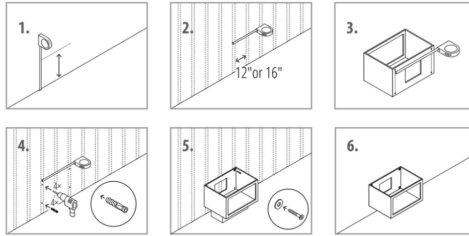
1. The recommended height of a wall mounted vanity is 32" to 34" inches above the ground. Measure a comfortable height according to your need and mark it on the wall.
