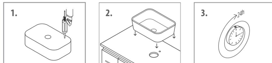
1. Add silicon glue to the back of the vessel sink.
