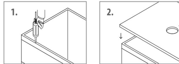
1. Apply continuous stream of quality silicon glue to the top of the cabinet where the countertop needs to be placed.
